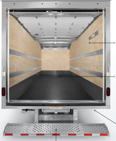
Plywood Liner with Steel Tie Bars
