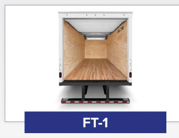
3/8" plywood sides, 1/2" plywood front for unobstructed cargo loading.
